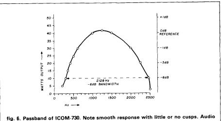
fig. 6. Passband of ICOM-730. Note smooth response with little or no cusps. Audio oscillator was swept over range of 200-2500 Hz.
